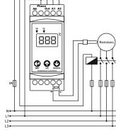
Marning: Pay attention to the polarities [+ & -] of NTC leads. Wrong connection may cause wrong measurement or sensor failure.
